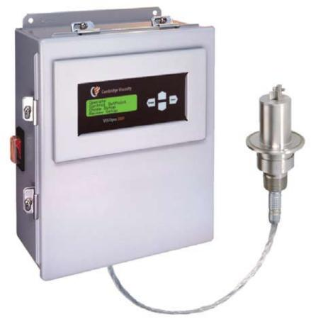
The VISCOpro 2000 viscometer offers menu-driven electronics to complement and control Cambridge Viscosity's high-quality in-line and in-tank sensors. Powerful yet easy to use, the VISCOpro 2000 provides viscosity, temperature, temperature-compensated viscosity, and optional density readings on an enhanced visual display panel. Thirteen factory-set standard measurement ranges from 0.2-20,000 cP are available for greater accuracy.
